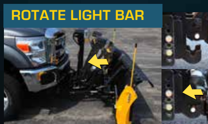
Moving light bar back causes mount pins to seat...
