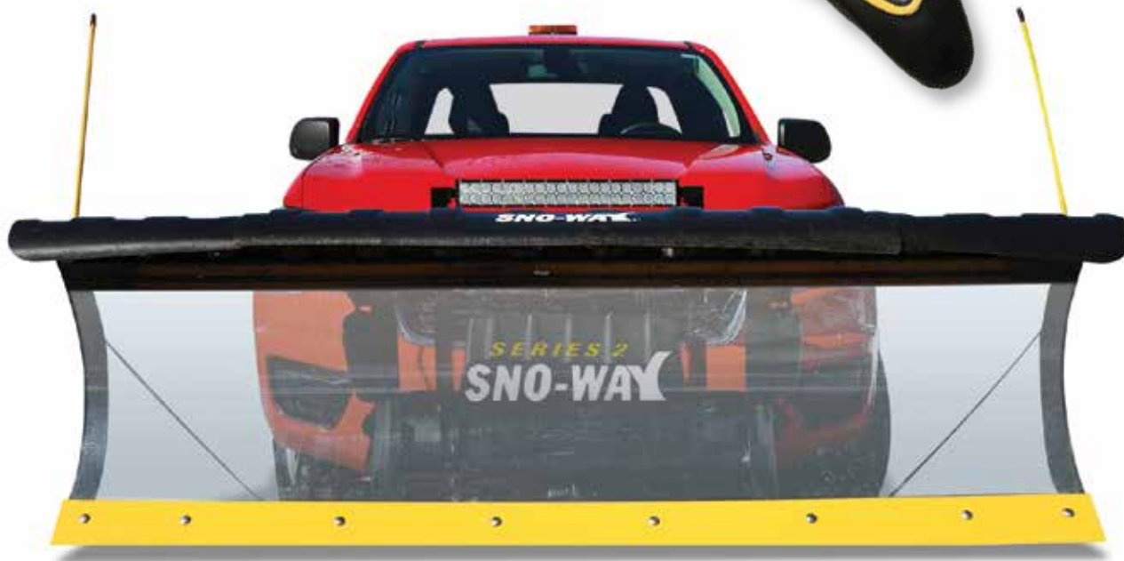
Driveway Series 2 blade shown with optional deflector and optional Smart Sight® Light
